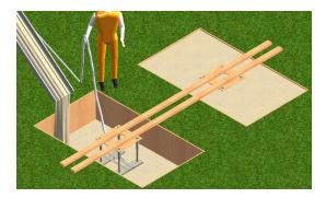
4. Immediately after concreting the bolt position and alignment should be rechecked to ensure the anchor has not moved.
